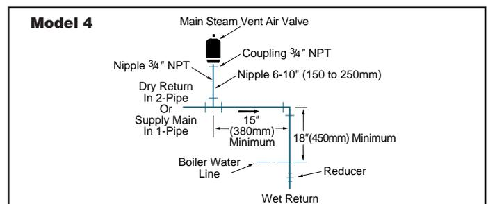
To prevent steam vents from sputtering water or damage from water hammer, observe the minimum elevations shown.
